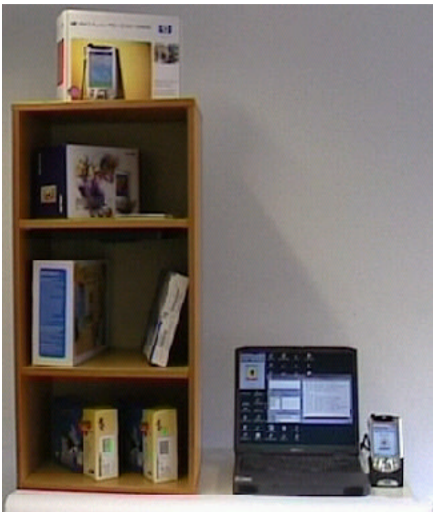
Figure 1: An environment for testing SPECTER with RFID input: an instrumented shelf with RFID-enriched products. On the right-hand side, a laptop which performs shop communication, and provides SPECTER with input. End-user display and interaction are performed via a PDA.
